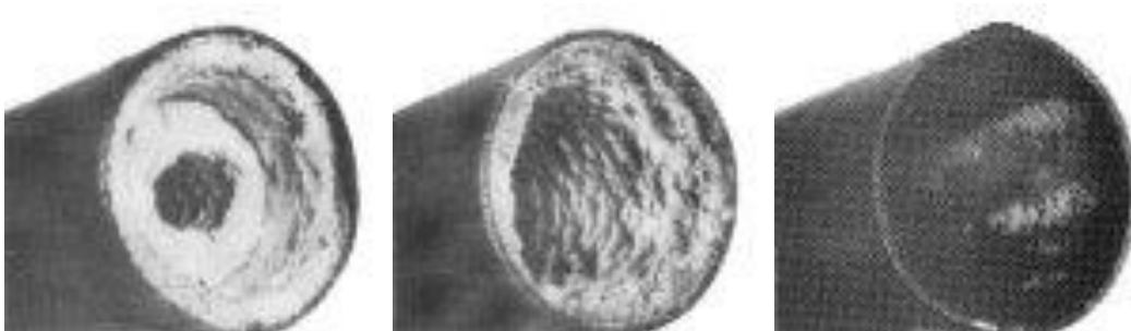
Before and after effects on calcium scale in pipes
